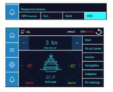
Operate stabilizers in At-Anchor mode while throttle is engaged at low speed.
