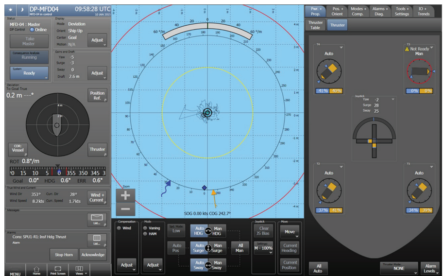
Dynamic Positioning - Working in conjunction with Shell Oil, Wärtsilä DP (as Honeywell) developed the very first DP systems ever constructed used for the Cuss 1 in 1961.
